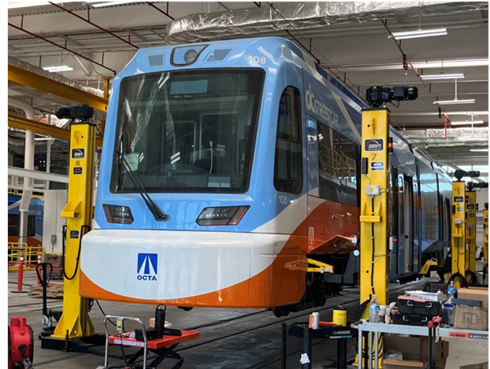
Vehicle Bumper Installation
