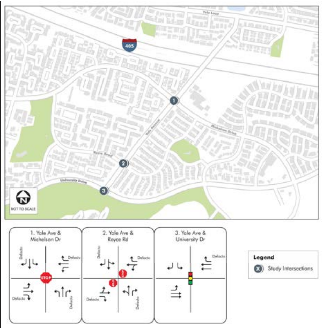
Figure 4-2: Existing Lane Configurations
