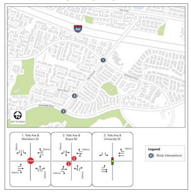
**Figure 4-2: Existing Lane Configurations**
