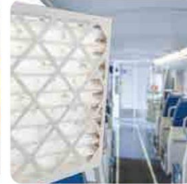
Antimicrobial air filters in train ventilation system
