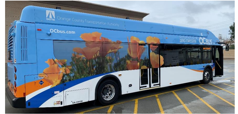
40-foot Hydrogen Fuel-Cell Electric Bus
