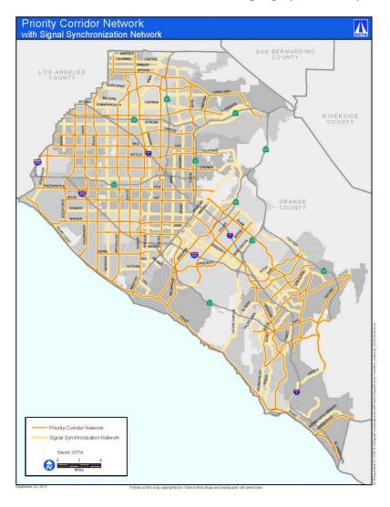
Under this focused effort, signalized intersections along each corridor will be upgraded to provide state of the practice intersection control and associated communications. Optimized timing plans will be developed and implemented along each corridor, aiding movement of the existing traffic patterns. This approach is considered essential to producing an optimized system as early as possible.
