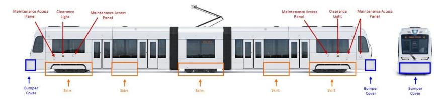
Highlighted areas prone to damage and therefore should be simplified in design and number of colors.
