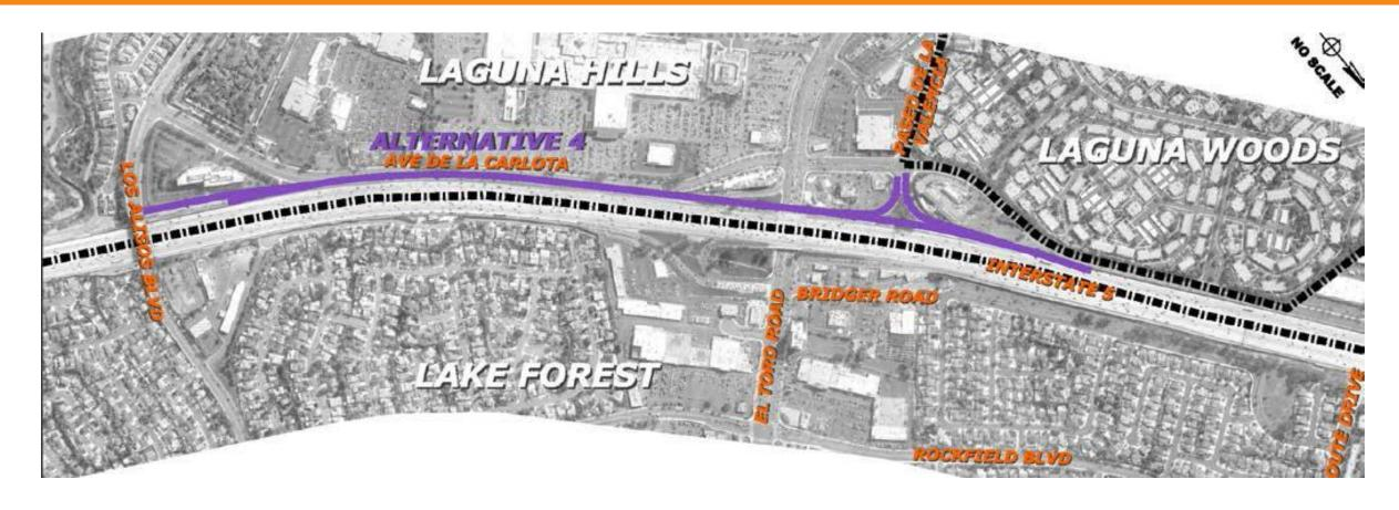
Southbound collector/distributer system from El Toro off-ramp to new Los Alisos Boulevard off-ramp
