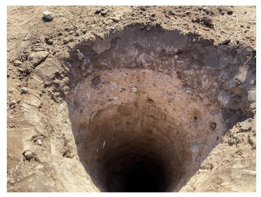
Figure 3. Soil profile at STP 36 showing layer of compacted fill beneath loose overburden
