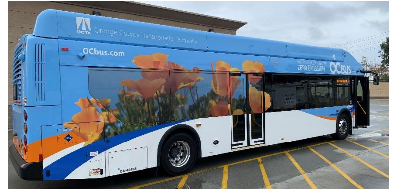
40-foot Hydrogen Fuel-Cell Electric Bus
