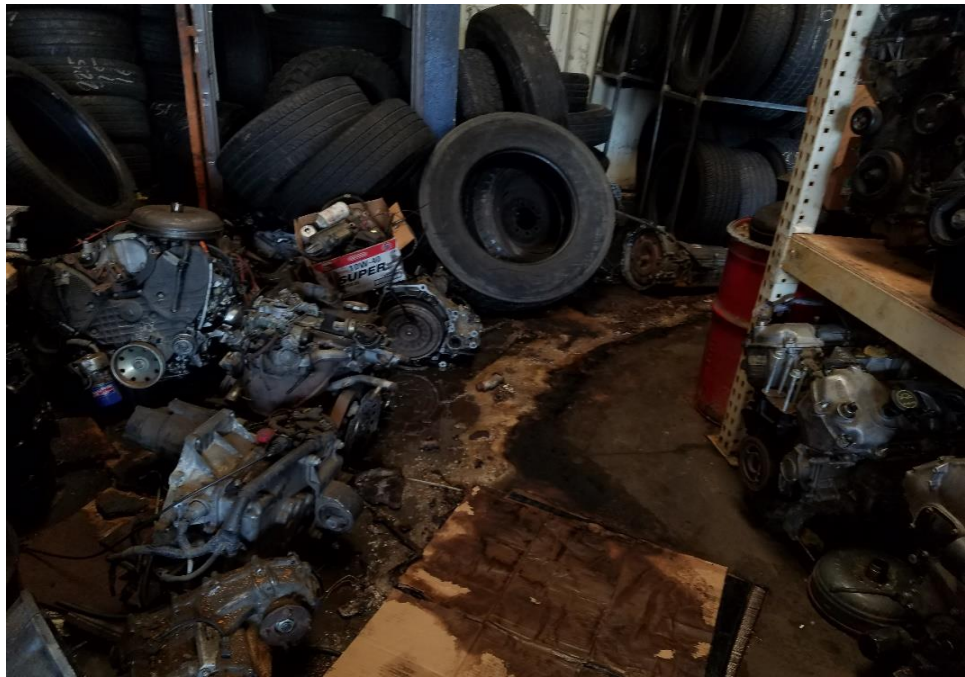
Photograph 14: View of oil staining located in Unit 1514.
