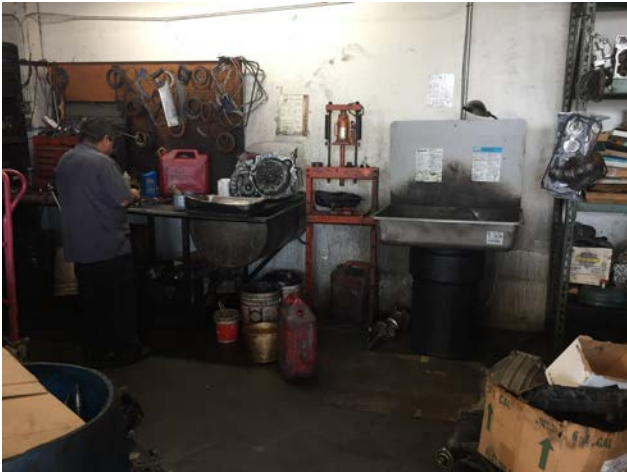
Photograph 4. View of the parts washer and the catch basin on the work bench in the California Japanese Auto Service unit.
